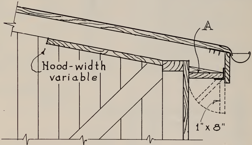
Fig. 17. Detail for constructing ventilators above rear-wall plate and between rafters. Baffle board is hinged at A . In some climates it is necessary to install a hood over the roosts to conduct air to center of house. Width of hood will vary with climatic conditions. Hood may be of fiberboard, plasterboard, or tongue-and-groove lumber.
